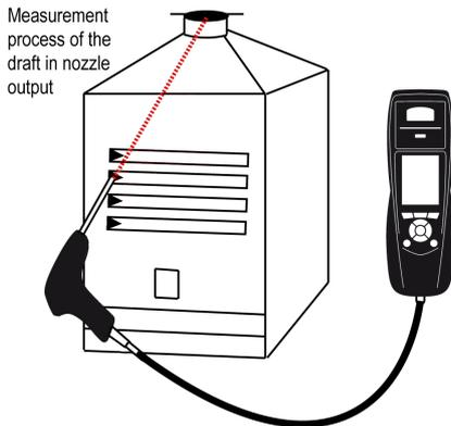
Put the probe of the KIGAZ 110 in the draft hood, going through the front face of the boiler
