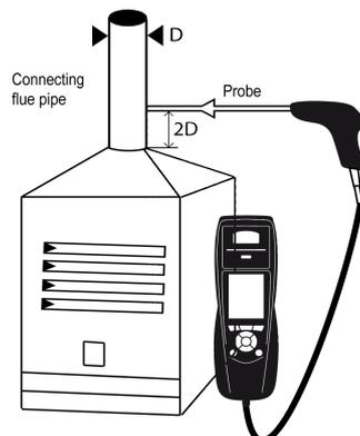
Put the probe of the KIGAZ 110 in the nozzle output, from the beginning of the connecting flue
