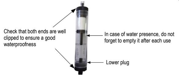
**! The presence of a water trap with filter can cause some gases solubility in water during gas analysis.**
